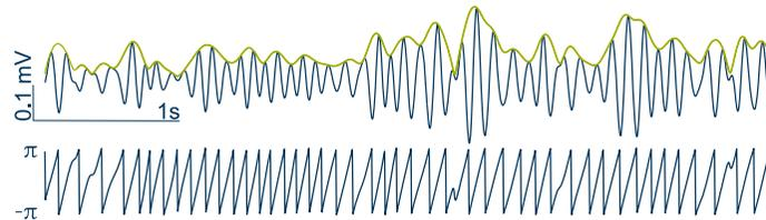
Figure 1: Based on the exemplary LFP that was filtered to the 8-12 Hz range (1st row, blue trace) the analytic amplitude, i.e., the signal envelope (1st row, orange trace) and the analytic phase (2nd row) can be derived using HT.
